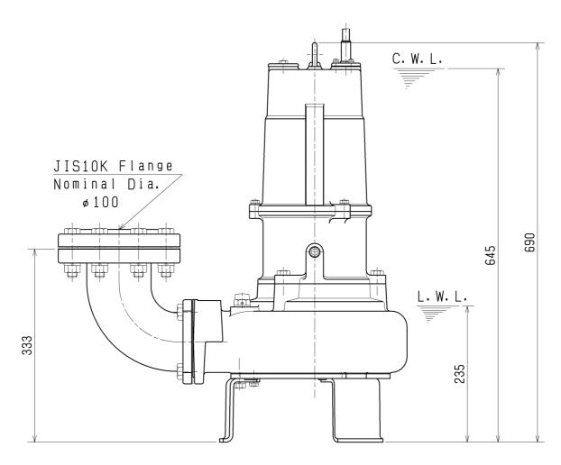
C. W. L. : Continuous runnning Water Level L. W. L. : Lowest runnning Water Level
