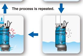
Pump stops in about one minute after the water level falls.
