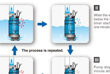
When the water surface falls below the electric probe, timer starts to count about
