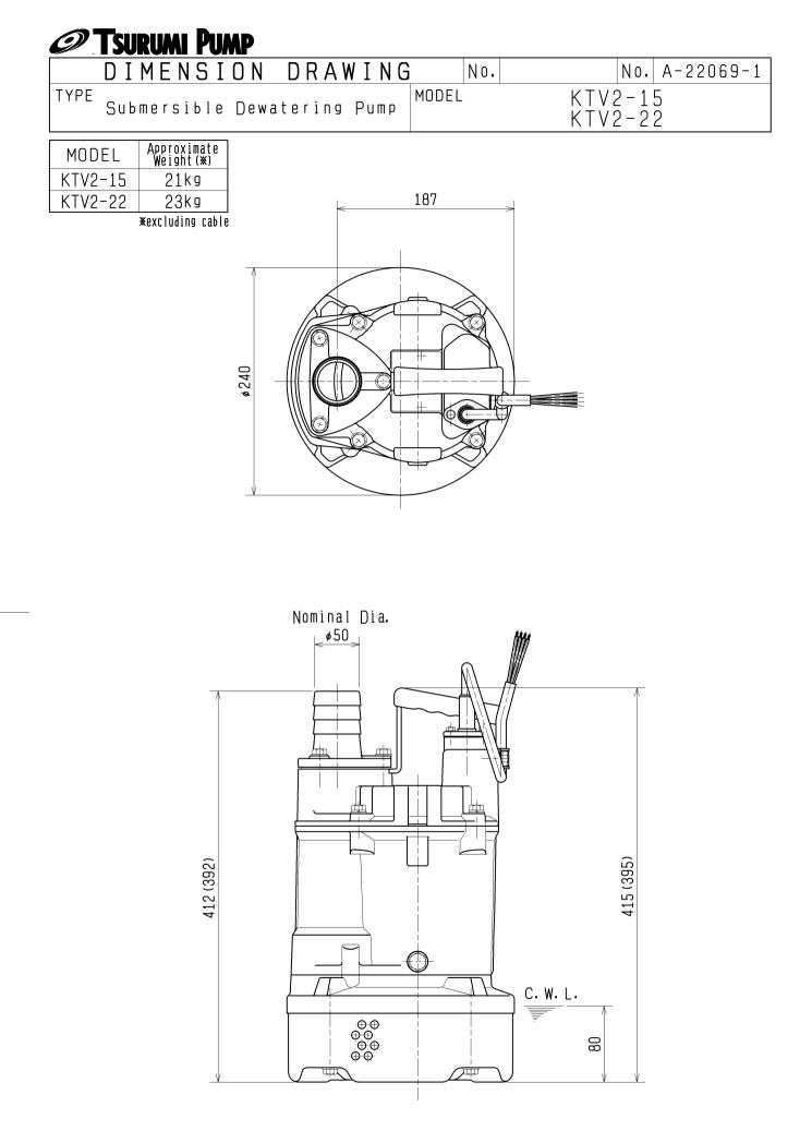
The Figure in ( ) shows the dimensions of KTV2-15. C.W.L.:Continuous running Water Level
